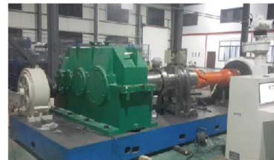
Yangzhou Hengchun 30W N.m electric actuator test bench 扬州恒春30W N.M电动执行器测试台
