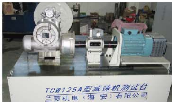
Jiangsu Sunshine TCW125A reducer test bench 江苏三上TCW125A减速机测试台
