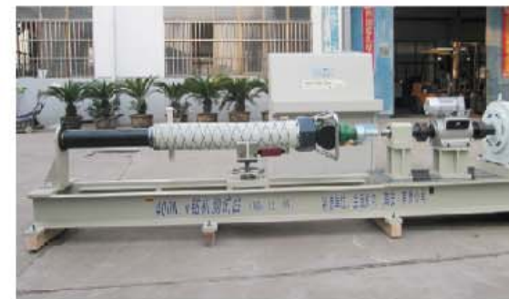
Jiangyin Zhongmei 400N.m drilling machine test bench 江阴中煤 400N.m钻机测试台
