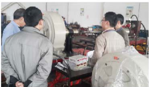
Nanjing Liuhe coal machine 5000N.m drilling machine test bench 南京六合煤机5000N.m钻机测试台
