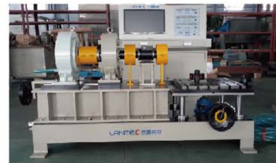
200N.m eddy current / magnetic series test bench 200N.m电涡流/磁粉串联测试台
