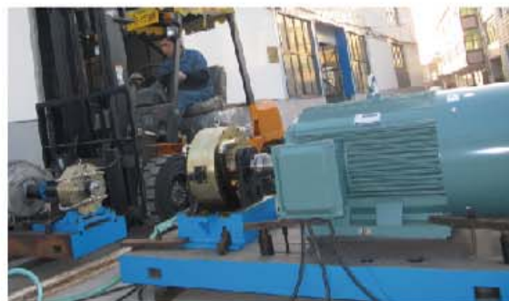
250KW, 40KW motor test bench 250KW、40KW电机测试台
