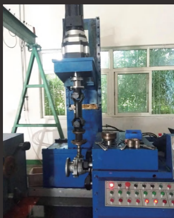
10kN.m阀门启闭扭矩测试台 10kN.m Valve opening and closing torque test bench
