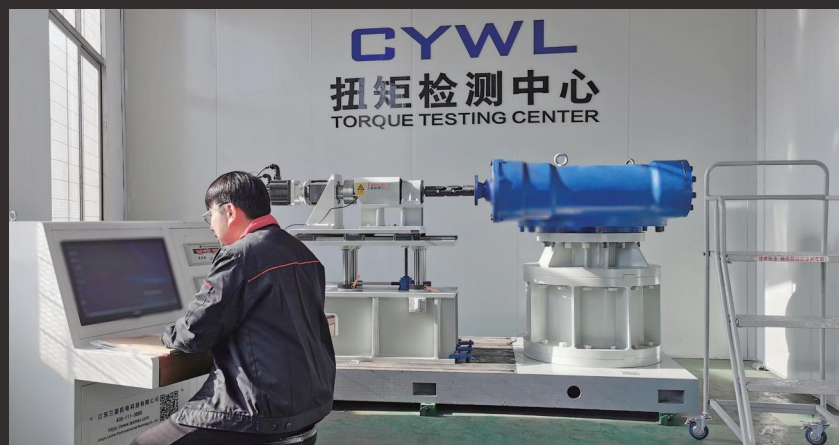
泉州超越300kN.m蜗轮箱测试台 Quanzhou Chaoyue 300kN.m Worm Gear Box Test Bench
