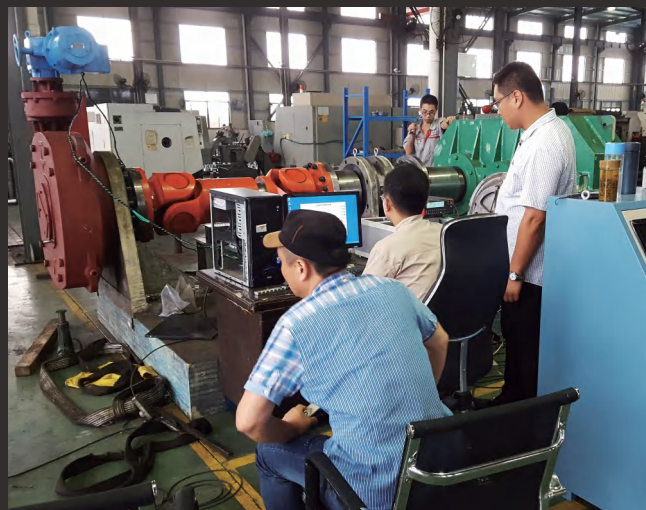
扬州电力修造厂 300kN.m蜗轮箱测试台 300kN.m Worm Gear Box Test Bench for Yangzhou Electric Power Equipment manufacture factory Co.,Ltd.
